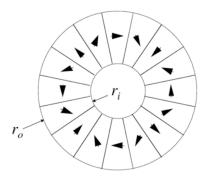
to calculate the magnetic field of this magnet, approximate the magnetization vector as a continuous function of  $\varphi$  as follows
