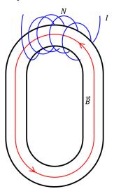
Each half of the electromagnet is of length L, so the circulation of **H** about this loop is
