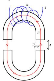
Note that for this part of the problem, we expect both B and H to be different in the electromagnet and in the gap. We will use B and H to describe the magnetic field in the electromagnet, and we will use  $B_{\rm gap}$  and  $H_{\rm gap}$  to describe the magnetic field in the gap.
