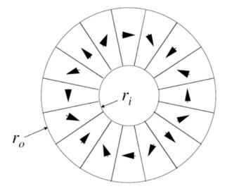
In order to calculate the magnetic field of this magnet, approximate the magnetization vector as a continuous function of  $\varphi$  as follows
