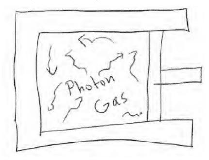
a) Consider a photon gas in a piston of volume V with walls in equilibrium with a reservoir at temperature T. Show that the energy density, U/V, is proportional to  $T^4$ . Hint: Consider the energies of the photon modes of a box and their occupation probability. Also you may use
