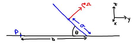
Let w be the angular velocity of the center of mass. If SL denotes the angular velocity of the disk about its center of mass then by equating the distance travelled by the point of contact we have
